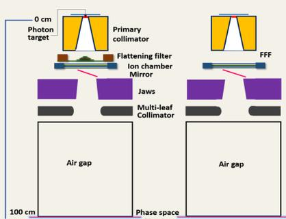
Fig. 3. the Varian Clinac linear accelerator treatment head. The right hand side of the figure shows the FFF linac parts.
