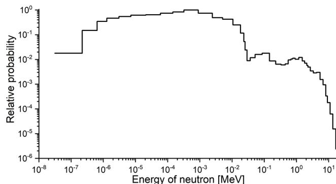
Figure 1: Energy spectrum of neutron beam from PuBe source. This data was also used for GATE simulation of neutron irradiation.
