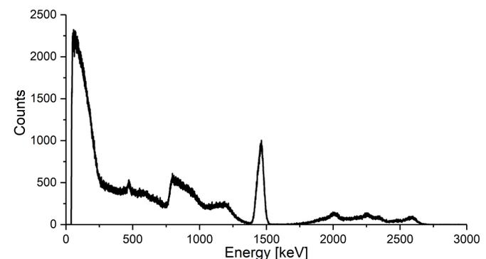
Figure 3: The energy spectrum of irradiated bone obtained by LaBr<sub>3</sub> detector measured by 1 week.
