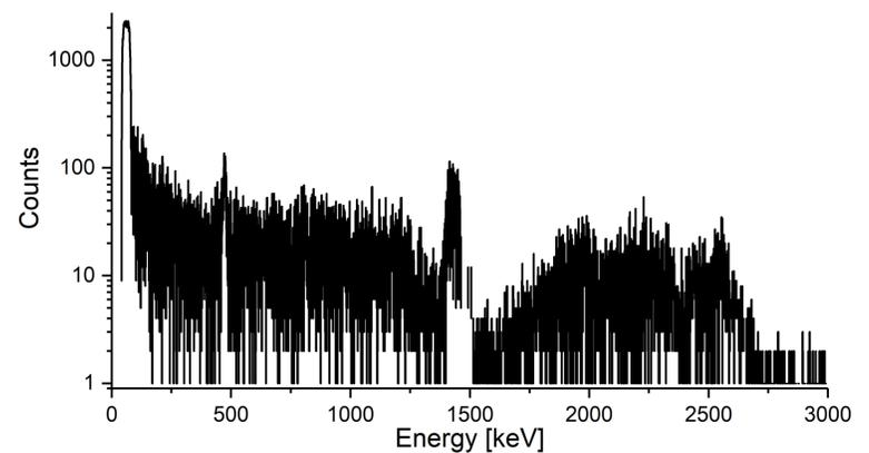
Figure 4: The energy spectrum of irradiated bone obtained by LaBr<sub>3</sub> detector with subtracted background radiation.
