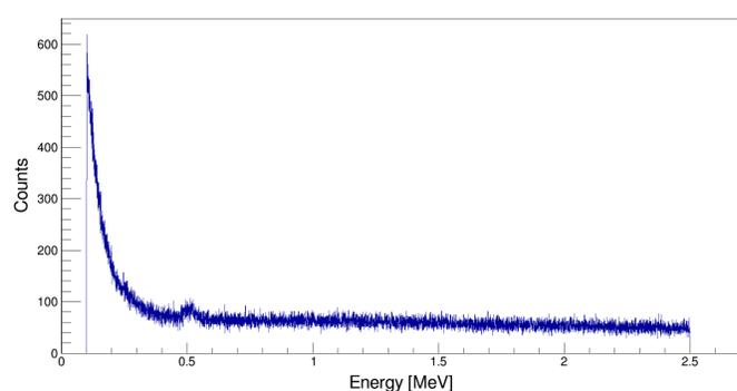
Figure 2: Gamma spectrum of the irradiated bone sample measured by NaI detector obtained by simulation. Irradiation calculated for  $2.5 \cdot 10^6$  neutrons. The energy spectrum measured by  $10^5$  seconds.
