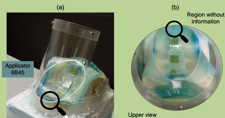
**Figure 1** – Sacral bone model with 3 film pieces of *Gafchromic* EBT3 : (a) Applicator 8B45 position and (b) applicator's upper view.
