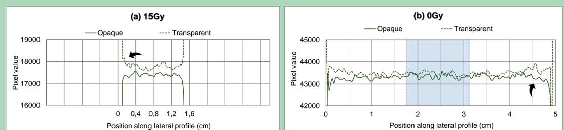
**Figure 4** – Transversal profile with templates of different opacities for a film irradiated with 15Gy (a) and an unirradiated film (b).
