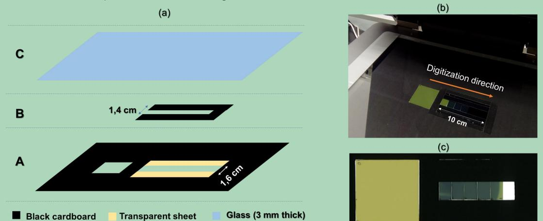
**Figure 3** – (a) Template placement scheme. **A**: black cardboard with acetate to place the reference and the irradiated film's samples; **B**: cardboard piece to minimize the signal lateral discontinuity; **C**: glass with 3 mm of thickness. (b) Example of the template placement in the scanner bed. (c) Image from an IOERT treatment where 5 film's samples were used.
