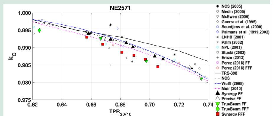
Fig 3. Beam quality correction factors for the NE2571 shown as a function of  $TPR_{20/10}$ . The large data points represents calculated values from the current study and the smaller data points are published measured  $k_Q$  factors. The solid black line represents data from TRS398 and the dashed black line is from the Dutch NCS protocol. The dashed magenta and blue lines are fits to Monte Carlo calculated values.
