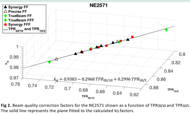
Fig 2. Beam quality correction factors for the NE2571 shown as a function of  $TPR_{20/10}$  and  $TPR_{10/5}$ . The solid line represents the plane fitted to the calculated  $k_Q$  factors.
