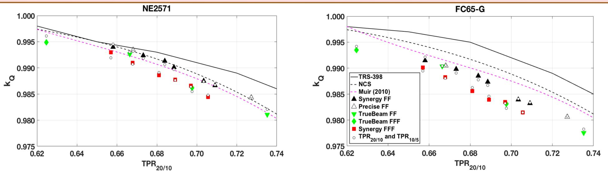
Fig. 1 Monte Carlo calculated  $k_Q$  factors for beams with flattening filter (triangles) and FFF beams (squares and diamonds) for NE2571 (left) and FC65-G (right). Open circles represents the bi-linear fit using  $TPR_{20/10}$  and  $TPR_{10/5}$ . Also included are fits from TRS-389, NCS and Muir et al. (2010).
