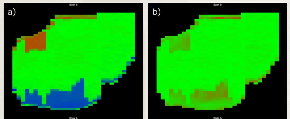
Figure 2: Fluence deviation of IMRT treatment due to position errors of MLC for a Varian Clinac. a) Color wash. b) Gamma evaluation.
