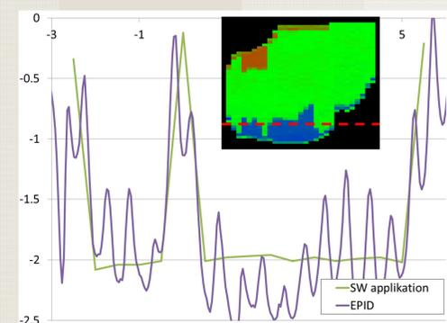
Figure 4: Comparison of the fluence deviation along the dotted red line measured with the EPID and the Treatment Delivery Tool.
