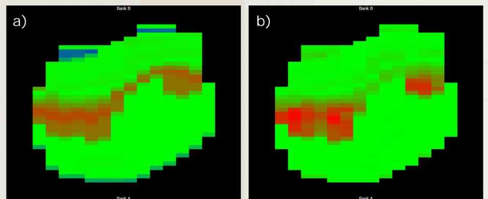
Figure 3: Fluence deviation of IMRT treatment due to a MU error for a Varian TrueBeam. a) Color wash. b) Gamma evaluation.
