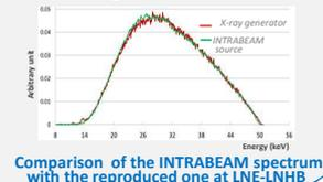
Comparison of the INTRABEAM spectrum with the reproduced one at LNE-LNHB
