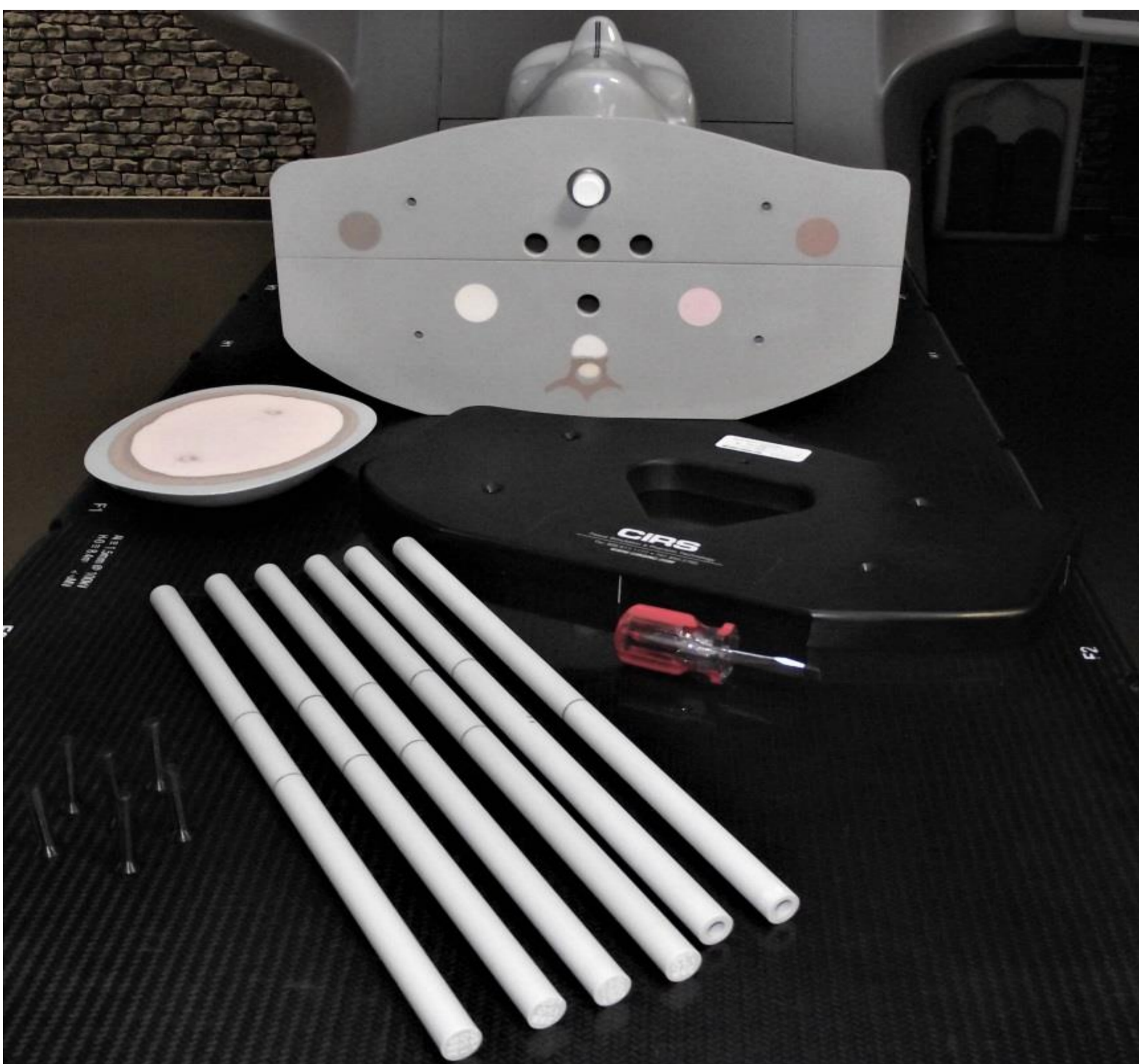
Disassembled CIRS SHANE with interchangeable sleeves for ionization chamber measurements in four longitudinal channels
