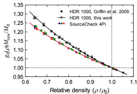
Figure 2. Normalized measured values, for Pd-103 source, corrected by the usual density factor,  $g_1(\rho)$ , as a function of the density ratio  $\rho/\rho_0$  for the three SourceCheck 4 $\pi$  ionization chambers (colored circles) and one HDR 1000 Plus chamber (squares) considered in the present work. The lines represent the fit of Eq. (3) to the data. Uncertainties are shown with a coverage factor  $k = 2$ .
