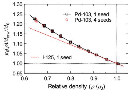
Figure 3. Normalized measured values, for Pd-103 source, corrected by the usual density factor,  $g_1(\rho)$ , as a function of the density ratio  $\rho/\rho_0$  for one of SourceCheck chamber when one (squares) or four seeds (red circles) are used. The dependence of this chamber for I-125 seeds is also shown (red dashed line). The Uncertainties are shown with a coverage factor  $k = 2$ .
