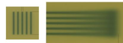
Gafchromic® films irradiated in the phantom using the collimator.
