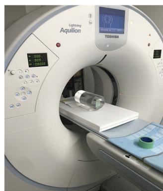
Fig. 3 Phantoms with Gafchromic film are on the bed of the CT.
