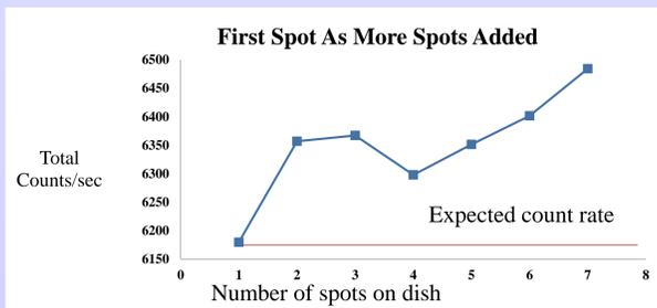
The IVIS was linear with time and activity when assessed for the full field of view. There was significant change in counts from a single sample as other samples were placed nearby. See graph. Reduction in light output was also observed as the sources evaporated with time but this was less than the increase from near by samples. Users need to consider cross talk between samples when imaging multiple samples.
