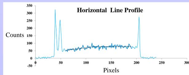
The horizontal line profile shows clear deviation in linearity. It appears to be less sensitive in the left side of Petri dish and became uniformly sensitive at the middle of the imaging. Several faulty or hot pixels were observed outside the sample area but these were unlikely to be the reason of the non-linear uniformity.
