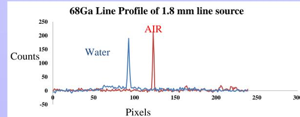
The optical resolution of the system is very high. The ability to image the radioisotope distribution depends on where the CR is generated. This is shown by the full width half maximum increasing from 1.86 in air to 2.29 when the line source was placed in water which allowed addition light to be generated outside the line source.
