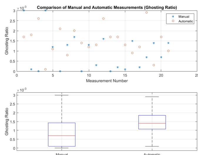
Figure 3. Comparison of variability in the measurement results between manual and automatic measurements, percent signal ghosting ratio test.
