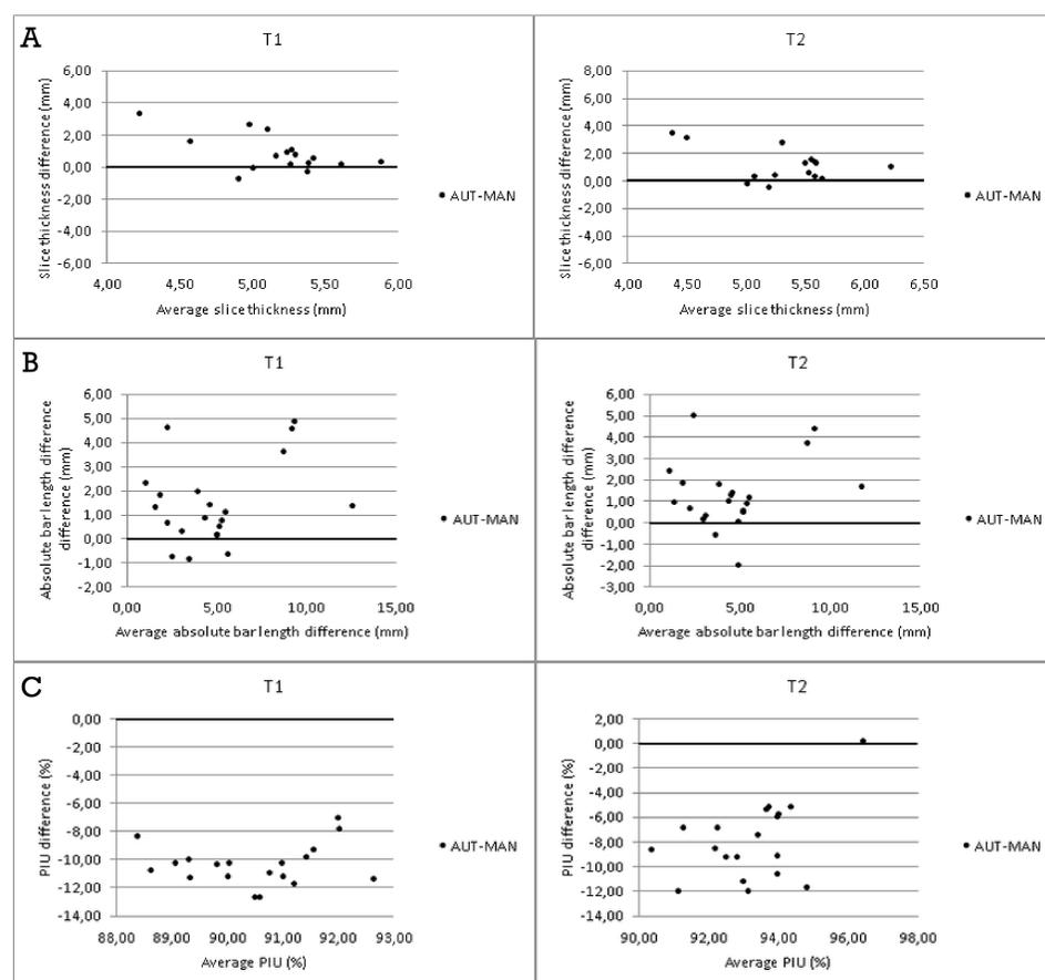
Figure 2. Difference between manual and automatic measurements in slice thickness accuracy (A), slice position accuracy (B) and image intensity uniformity (C) tests.
