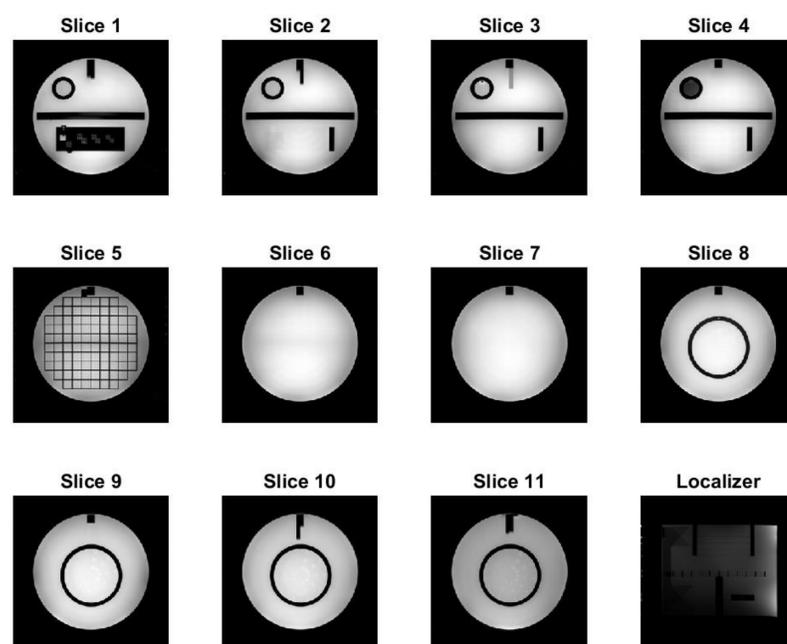
Figure 1. Image of the T1-weighted ACR phantom series and a localizer image from the ACR quality control protocol.
