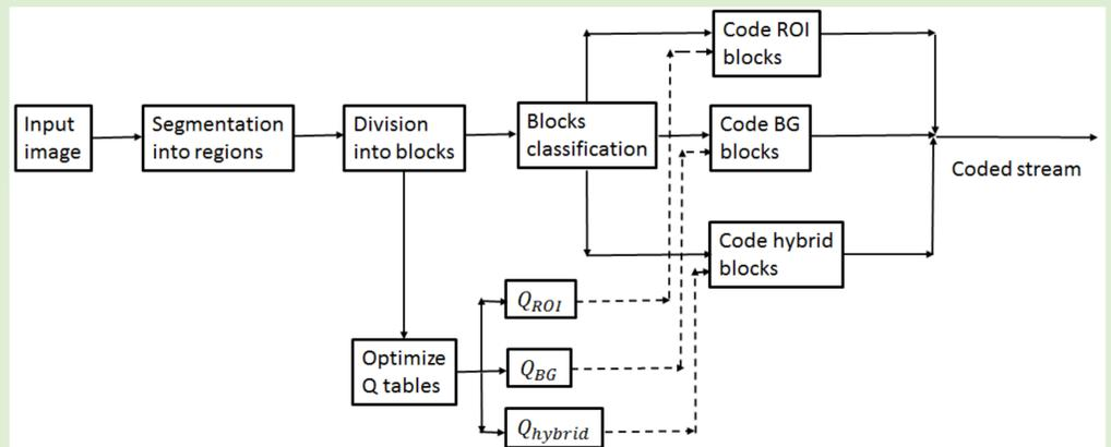
Figure 2 – Block diagram for the proposed coding algorithm.
