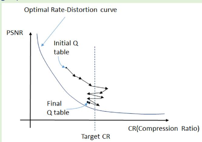
Figure 1 – Convergence of the iterative algorithm for optimization of the Q-table.
