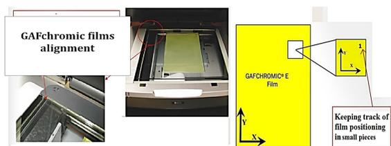
Figure 2. Film alignment using scanner and small piece track of film positioning
