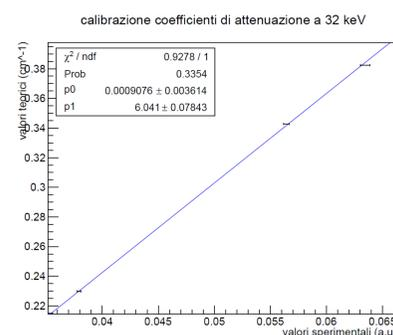
Fig 2. Example of calibration at 32 keV and MGD of 5 mGy. Three reference materials (ethanol, water and glycerol) are used. Theoretical values are taken from [5] while experimental values are evaluated, for each sample, as the average signal intensity, over several slices, of homogeneous ROIs. One sigma error bars.
