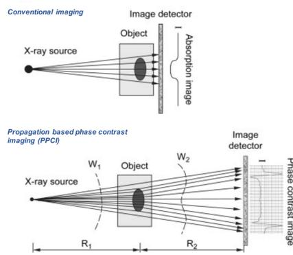
Fig 1. Conventional imaging compared to propagation based phase contrast imaging. In PPCI the detector is not placed just behind the object and the beam freely propagates before being detected. As a result, the edges of details are enhanced. From [2].
