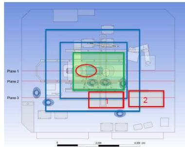
The C-arm is blocking the laminar airflow causing air to stagnate and even turbulence underneath the obstacle. Contaminations are not pushed away, so there is no cleaning effect of the LAF. Moreover critical areas outside the central area are not protected.
