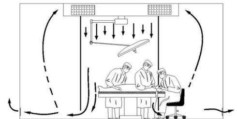
If Charnley's principle is not fulfilled, CFD calculation is necessary. The Halton Vita OR Space solution gives good air quality even in complex OR (ceiling-mounted devices, multiple critical zones).
