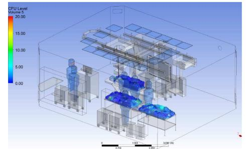
This paper presents the results of a comprehensive simulation of the solution in operation conditions. The simulation confirmed that even for very complex procedures, the studied solution is capable of producing ultra clean (<10 CFU/m<sup>3</sup>) conditions according to CEN TC156 WG18 standard draft EN 16244-2. Moreover this has been accomplished at a maximum 40 dBA ventilation system sound level.
